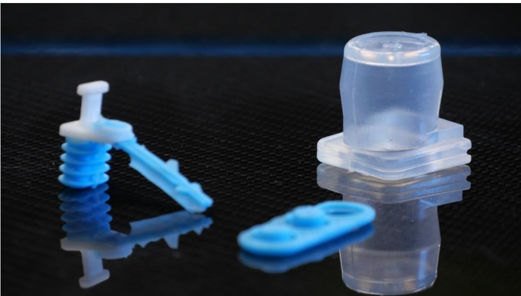
Cast silicon parts created via Figure-4 moulds
