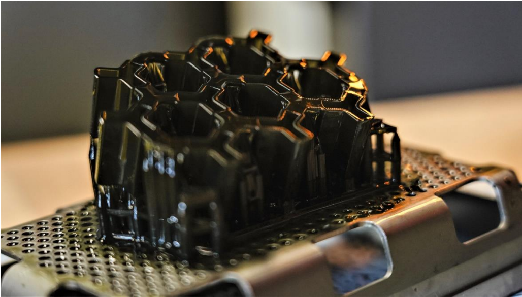
Support material on a part removed from the Figure-4
