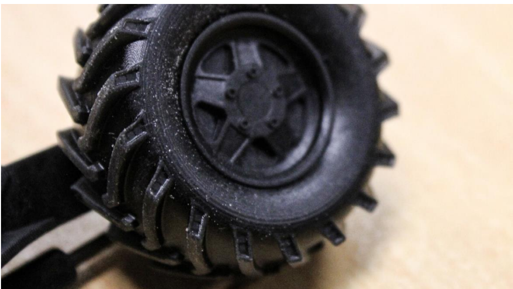
A multi-material assembly printed with Pro-Black and Rubber on the Figure-4
